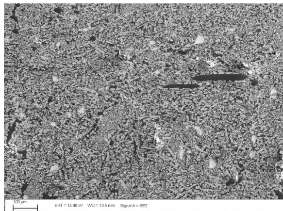
Acetylene black containing battery plate – raw (left side) and formed (right side). Carbon particles are well distributed and not generally visible within the structure. There are some regions which appeared more porous, which may be the result of large agglomerates of carbon particles, as illustrated previously for the carbon itself prior to incorporation in the negative active material.
