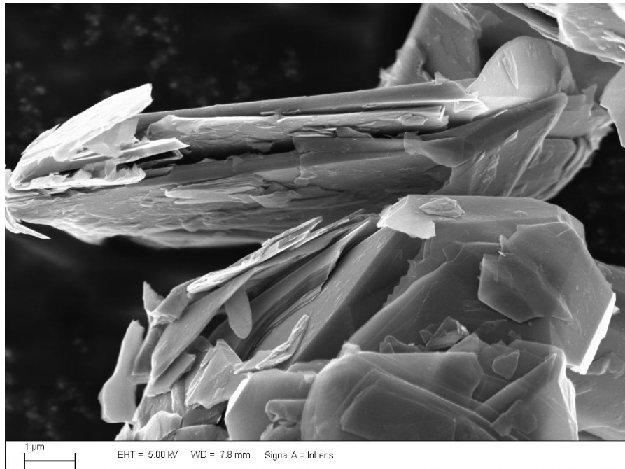
SEM image of the natural graphitic material. The material consists of numerous plates of graphitic carbon, as expected for such materials.
